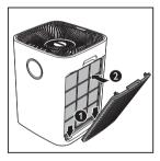
Repeat the above steps and assemble the filter for the other side of the appliance.
