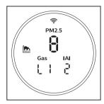
3 Touch and hold the  $\circlearrowleft$  button for 3 seconds to switch off the air purifier.
