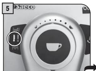
The indicator light starts flashing. Wait until the indicator is permanently on.
