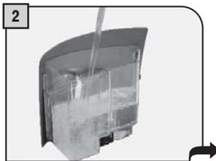
Empty the tank and refill it, dissolving the descaling solution in a full tank of water.
