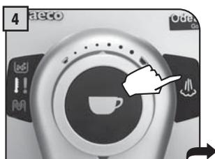
Press the button to select the steam function. The steam light turns on.
