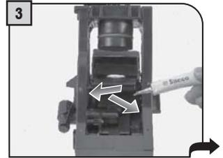
3 Lubricate the brew group guides using the supplied grease only.
