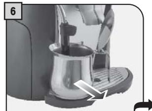
Empty the container with the used descaling solution.
