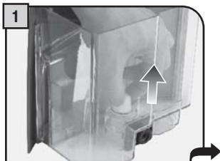
Remove the small white filter from the water tank and store it in a dry place sheltered from dust.
