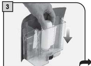
Insert the filter in the empty tank. The reference mark and the groove must match. Push firmly until it is completely inserted.
