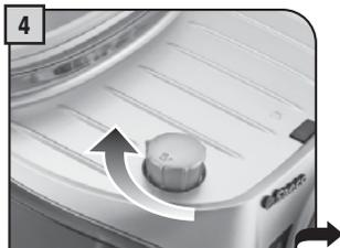
Turn the knob until the
