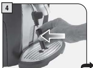
Remove and wash the steam/hot water wand. Wash all external components.
