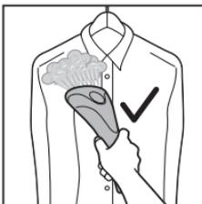
**EN** Do not use the appliance on an ironing board, at a low position where the hose forms a U-shape, or hold the steamer head upside down. Otherwise condensation in the hose cannot flow back into the water tank. This may cause irregular steam, water dripping from the steamer head and/or a croaking sound.
