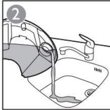
**EN** Always empty the water tank after use, to prevent scale build-up. Rinse the water tank to remove any deposits.
