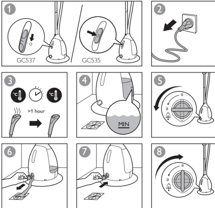
**EN** To maintain optimal steam performance, it is important to remove scales and impurities inside the appliance regularly. Therefore, it is recommended to perform the easy rinse calc-clean process at least once a month. Before you start calc-clean, make
