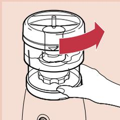
**6** When you have finished chopping, switch the appliance off, unplug it and detach the chopper by turning it in the direction of the arrow.
