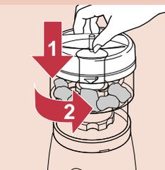
**4** Put the lid on the bowl, push it down and turn it in the direction of the arrow until it is entirely fixed. Make sure it is properly fixed before you switch the chopper on.
