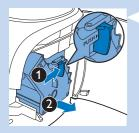
4 Press the PUSH button (1) and pull at the grip of the brewing unit (2) to remove it from the machine.
