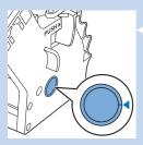
7 Before you slide the brewing unit back into the machine, make sure the two reference signs on the side match. If they do not match, perform the following step:
