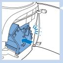
9 Slide the brewing unit back into the machine along the guiding rails on the sides until it clicks into position.
