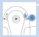
The descaling light and the on/off button light up continuously. You have to descale the machine. Follow the instructions in chapter 'Descaling the machine'.
