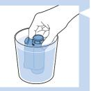
2 Remove the filter from its packaging and immerse it in cold water with the opening pointing upwards. Press the sides of the filter gently to let out the air bubbles.
