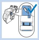
8 Make sure the locking hook of the brewing unit is in the correct position.
