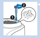
1 Press the grinding degree adjustment knob firmly (1) and then turn it one notch at a time (2). There are 5 different grinding degree settings you can choose from. The smaller the dot, the stronger the coffee. The difference becomes noticeable after you have brewed 2-3 cups of coffee at the new setting.
