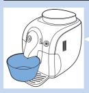
When the machine has heated up, it performs an automatic rinsing cycle to clean the internal circuit with fresh water. This takes approximately one minute
