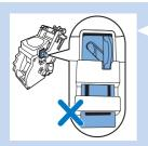
Note: The hook is not correctly positioned if it is still in bottommost position.
