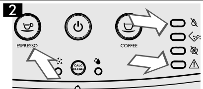
"☕" steady on "⌵" and "⚠" flashing
