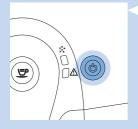
Note: If you want to interrupt the water flow press the coffee button. To restart the water flow, press the coffee button again.
