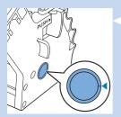
7 Before you slide the brewing unit back into the machine, make sure the two reference signs on the side match. If they do not match, perform the following step:
