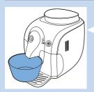
During the initial heat-up process, fresh water flows through the internal circuit to heat up the machine. This takes a few seconds.
