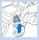
To position the hook correctly, push it upwards until it is in uppermost position.
