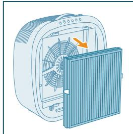
2 Pull the downside of the front cover out from the appliance and lift it upwards.
