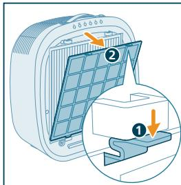
3 Remove the purification filter from the appliance.
