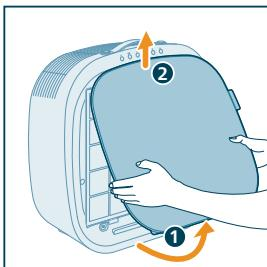
2 Press the clips on the both sides of the pre-filter to remove it.
