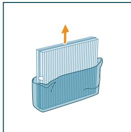
7 Put the Integrated HEPA and Active Carbon filter back to the appliance, ensuring that the filter with two clips is facing outwards.
