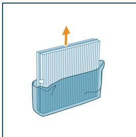
6 Put the pre-filter back to the appliance. Make sure you insert the pre-filter into the left and right holes at the bottom side. The two clips on the top of the filter make a "click" sound when installed properly.
