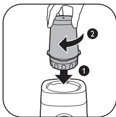
3 Turn the assembled beaker clockwise to lock it to the motor base.
