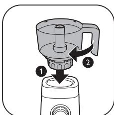
**2** Turn the assembled chopper bowl clockwise to lock it to the motor base.
