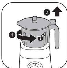
9 Turn the grinder jar anti-clockwise to remove it from the motor base.
