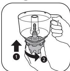
**1** Turn the coupling unit anti-clockwise to lock it to the chopper bowl.
