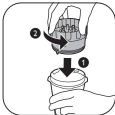
2 Turn the mill blade unit anti-clockwise to lock it to the beaker.
