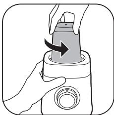
9 Turn the mill blade unit clockwise to remove it from the beaker.
