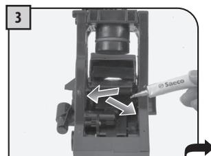
Lubricate the brew group guides using the supplied grease only.
