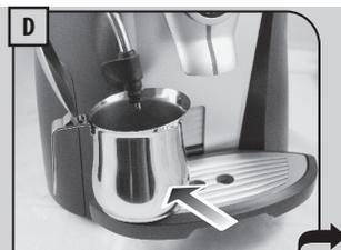
If descaling solution spills out of the steam wand: Pause: turn the selector switch to the
