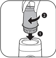
**3** Turn the assembled beaker clockwise to lock it to the motor base.
