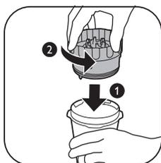
**2** Yanchish mashinasining pichoq blokini o'lchash stakaniga mahkamlash uchun blokni soatga qarshi buring.
