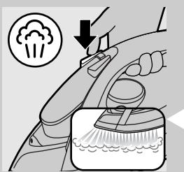
The forward-directed concentrated shot of steam enhances the distribution of steam into every part of your garment. The concentrated shot-of-steam function can only be used at temperature settings between ●● and MAX.
