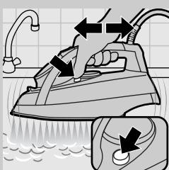
Steam and boiling water will come out of the soleplate. Impurities and flakes (if any) will be flushed out.
