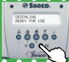
When the machine gives the signal, press the button x 5 seconds.
