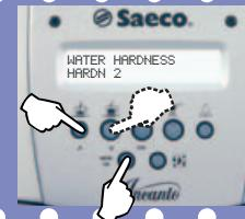
Select the corresponding hardness (e.g. 2 squares = Hardness 2) and memorize the value by pressing the "OK" button.
