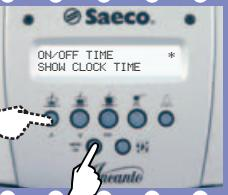
Menu for programming machine ON/OFF times.
