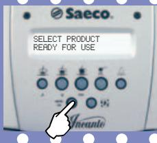
Press the "OK" button to restore the machine to normal operation.
