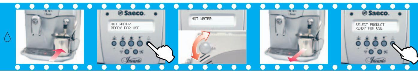
Place a container beneath the steam tube.
