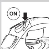
**4** Press the Ionic DeepSteam button once to switch on the Ionic DeepSteam function.
