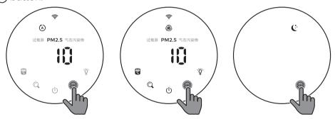
**Auto mode ( (A) ):** In Auto mode, the dual-sensor senses the air quality in real-time and the appliance automatically adjusts the fan speed in accordance with the ambient air quality.
