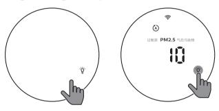
With the light sensor, the control panel can automatically turn on, turn off or dim according to the ambient light. The control panel will be off or dim when the ambient light is dark. You can touch any button to wake up all lights. Then, if no further operation, all lights will be off or dim again to match with the ambient light.
