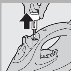
**6** Hold the iron over the sink and set the steam control to position ● (Calc-Clean). The steam control knob will spring up slightly.
