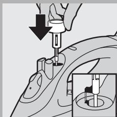
**9** Use vinegar to remove scale, if any, from the needle.
