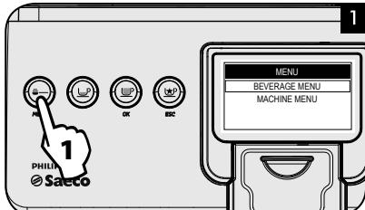
**EN** Press and hold the button for 5 seconds.
