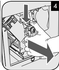
**EN** Remove the brew group: Pull it by the handle and press the «PRESS» button.
