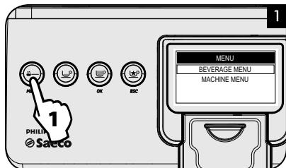
Press and hold the button for 5 seconds
