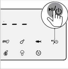
2 Press the On/Off button again to turn on the device.
