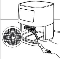
**5** Clean the heating element with a cleaning brush to remove any food residues.
