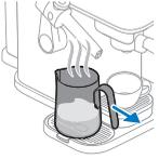
**8** While the machine is brewing coffee, remove the jug with milk froth from the machine.
