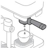
**8** The machine heats up and starts rinsing water from the coffee spout into the cup. The Intensity boost button will continue to blink slowly during this process.
