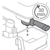
**6** The machine dispenses the entire descaling solution at regular intervals through the coffee spout and smart foam wand alternately. This takes up to 30 minutes.
