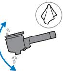
**10** Shake off excessive water from the portafilter and dry the portafilter with a cloth. The machine is now ready for use.
