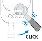
The direct start function allows you to switch on your machine and brew delicious coffee easily or start frothing. There is no on/off button. Simply press the button of the drink you want to brew and move the portafilter to the right to start grinding and brewing. After pressing the Foam button, the machine will heat up and start steaming automatically.
