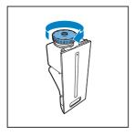
5 Shake the bucket to and fro with both hands to clean the inside of the water bucket.
