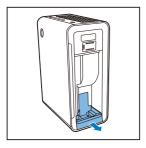
4 Remove the humidification filter from the humidification filter tray.
