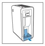
Remove the humidification filter from the humidification filter tray.
