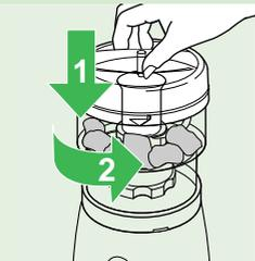
**4** Put the lid on the bowl, push it down and turn it in the direction of the arrow until it is entirely fixed. Make sure it is properly fixed before you switch the chopper on.
