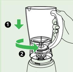
**3** Mount the jar unit onto the motor unit. Fix it by turning it in the direction of the arrow.
