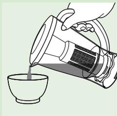
**7** Switch the appliance off and remove the blender jar from the motor unit. Pour out the drink through the spout of the blender jar.
