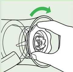
**2** Attach the knife unit to the blender jar by turning it in the direction of the arrow.
