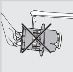
Do not clean the filter cylinder case with the filter cylinder in it under the tap.
