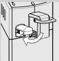
**2** Push the water dispensing spout towards the bottom while rotating it at the same time, until it is locked in the machine as shown in the figure.
