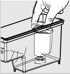
**4** Put the "INTENZA+" water filter into the empty water tank. Press it down until it cannot move any further.
