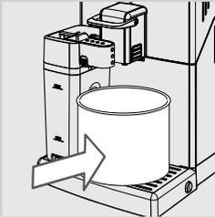
**16** Insert the milk carafe into the machine. Pull out the milk carafe dispenser to the right up to the “☕” icon. Place a container under the dispensing spout to start the rinse cycle.
