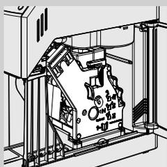
**13** After rinsing the brew group, insert it back into its seat until it locks into place (see the “Weekly Cleaning of the Brew Group” chapter). Insert the drip tray and the coffee grounds drawer. Close the service door.
