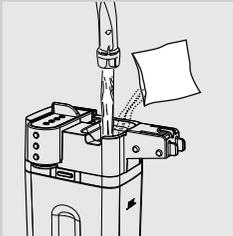
**1** Fill the milk carafe with water up to the maximum level (MAX).
