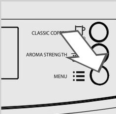
**5** Press the "☰" button. The machine shows this display.
