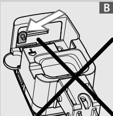
**16** If you cannot install the dispenser at the top of the carafe, the pin is in the wrong position (B). Before installing the dispenser, manually push the pin to the (A) position.
