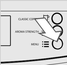
5 Press the “☰” button. The machine shows this display.
