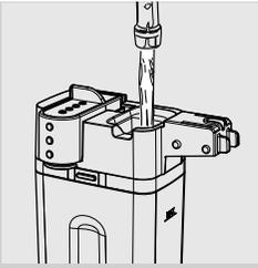
**4** Remove the lid and fill the milk carafe up to the MAX level with fresh water.
