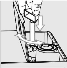
**4** The reference marks inside the coffee bean hopper indicate the grind setting. There are 5 different grind settings to choose from, from position 1 (●) for coarse grind - lighter taste to position 2 (●) for fine grind - stronger taste. If coffee is watery or is brewed slowly, change the coffee grinder settings.
