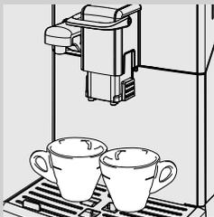
Two cups can also be placed under the dispensing spout to brew two cups of espresso or long espresso at the same time.
