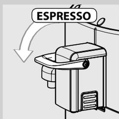
Before brewing beverages as described below, the lever must be rotated to the correct position.
