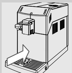
**16** Insert the coffee grounds drawer with the drip tray back into the machine and close the service door.
