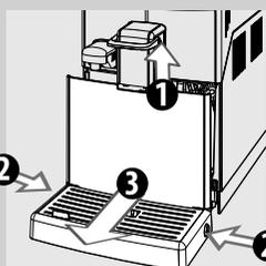
**17** To clean the drip tray, place a “Coffee Oil Remover” tablet inside and fill it 2/3rds full with hot water. Let the cleaning solution take effect for about 30 minutes, then rinse thoroughly.
