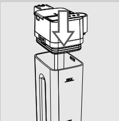
**18** Attach the top of the milk carafe, ensuring it is locked into place.
