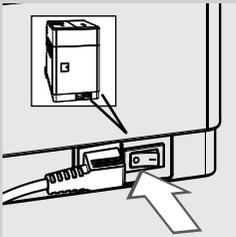
**8** Switch the power button on the back of the machine to “0”.
