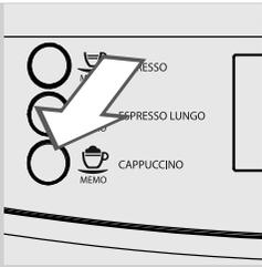
**4** Press and hold the “MEMO” button until the “MEMO” icon appears on the display. Then release the button. The machine is now in programming mode.
