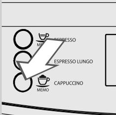
**5** Beverage brewing automatically stops when the pre-set level is reached; press the “☕” button to stop it earlier.
