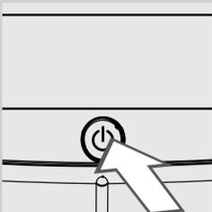
**10** Switch the power button on the back of the machine to “I”. To turn on the machine, press the “⏻” button. Wait until the end of the automatic rinse cycle.
