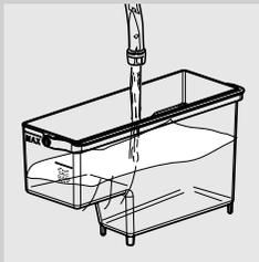
**15** Remove the water tank, rinse it and fill it with fresh water up to the CALC CLEAN level. Put it back into the machine.
