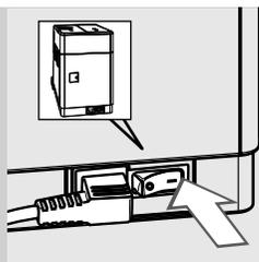
**12** Switch the power button to "I". The "⏻" button flashes.
