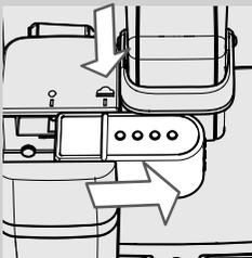
**3** Insert the carafe into the machine. Pull out the milk carafe dispenser to the right up to the “
