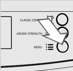
**4** Press the "☰" button. The machine shows this display.
