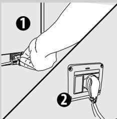
**10** Insert the plug into the socket located on the back of the machine.
