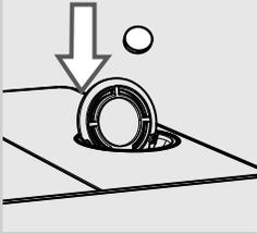
**3** Put a “Coffee Oil Remover” tablet in the pre-ground coffee compartment.
