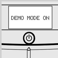
The machine is provided with a demo program. By keeping the "⏻" button pressed for more than 8 seconds, the machine enters the demo program. Turn the machine off and on again using the power button to exit the function.
