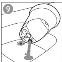
**EN** Calc cleaning removes scale and impurities trapped inside the steamer after prolonged use. We recommend calc cleaning every month. If necessary, repeat the steps for more thorough cleaning. Make sure there is some water in the water tank before you start calc cleaning.
