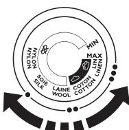
**3** To set the required ironing temperature, turn the temperature dial to the appropriate position (see the 'Temperature and steam settings' table above).
