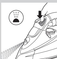
You can use the spray function at any temperature to moisten the article to be ironed. This helps remove stubborn creases.
