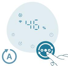
**Sleep mode (
