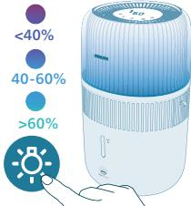
You can press the button to turn on humidity light, ambient light or turn off all lights and the control panel.
