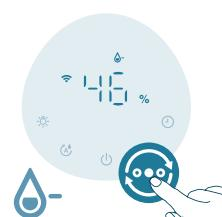
**High mode (
