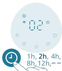
Press the timer button repeatedly to choose from 1, 2, 4, 8 or 12 hours. Once the timer ends, the humidifier will stop operating automatically.
