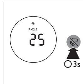
A diagram showing a circular control panel with a central display showing "PM2.5" and "25". To the right of the panel is a larger circle containing a padlock icon, with a hand icon pointing upwards and a timer icon below it labeled "3s" to indicate a hold action.
