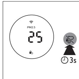
A diagram showing a circular control panel with a central display showing "PM2.5" and "25". To the right of the panel is a larger circle containing a crossed-out padlock icon, with a hand icon pointing upwards and a timer icon below it labeled "3s" to indicate a hold action.
