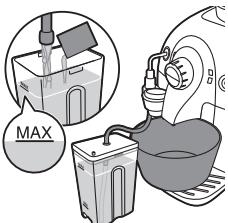
Cleaning cycle with milk circuit cleaner and water.
