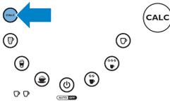
11. Press the CALC button to start the flushing cycle. The water flows continuously for approximately 5 minutes.
