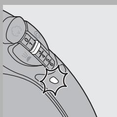
**3** Put the mains plug in an earthed wall socket. The temperature light goes on to indicate that the iron is heating up.
