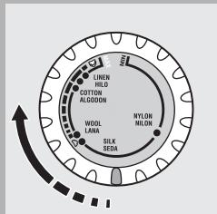
**2** Set the required ironing temperature by turning the temperature dial to the appropriate position (see section 'Tips' for extra information).
