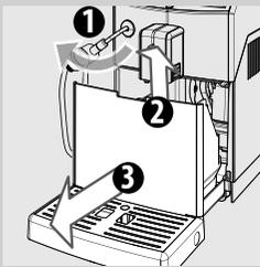
**16** To clean the drip tray, place a “Coffee Oil Remover” tablet inside and fill it up to 2/3rds full with hot water. Let the cleaning solution take effect for about 30 minutes, then rinse thoroughly.
