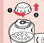
1 To attach the blender jar, remove the screw cap above the panel.
