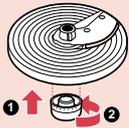
**2** Connect the knob from the bottom side of the disc and turn it to position dot to lock it.
