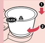
**2** Place the mixing bowl on the motor unit and turn it into the direction of the arrow until you hear a 'click'.
