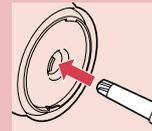
**1** Push the driving shaft of the mixing bowl into the opening of the mixing bowl from below. You will hear a 'click' when it snaps into place.
