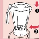
2 Mount the blender jar on top of the motor unit by turning it in the direction of the arrow until it is firmly fixed. The handle must be facing to the left!
