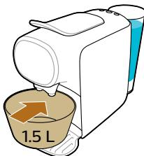
5 Place a bowl with a minimum capacity of 1.5 liters on the lower drip tray under the coffee dispensing spout to collect the descaling solution.
