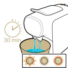
7 The machine dispenses the entire descaling solution at regular intervals. This takes up to 30 minutes.
