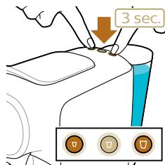
6 Press and hold the ristretto and lungo button for 3 seconds at the same time. The ristretto button starts to flash and the lungo button is steady on
