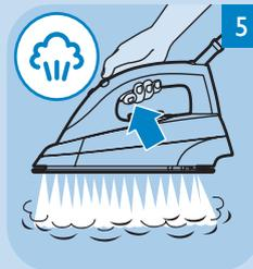
**5** If you want to iron with steam, set the temperature dial of the iron to ●● or higher and press the steam activator **T**.
