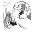
**7** Clean the coffee exit duct thoroughly with the provided tool. Insert it as indicated in the figure.
