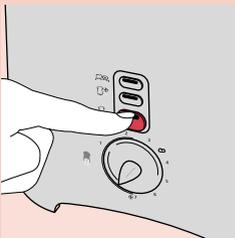
**5** Select the desired browning setting, push the toasting lever down to switch the appliance on and press button **Q**.
