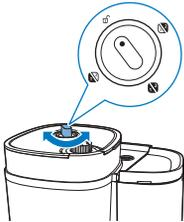
8 Turn the container selector knob to choose desired beans between the two containers.
