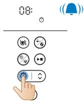
4 Press the timer button to confirm the hour setting. The minutes digits indicate setting minute.
