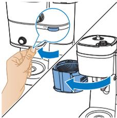
5 Place the filter in the filter basket and close the filter basket holder.
