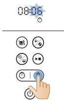
5 Use the arrow button again to adjust the minutes. If you need to adjust quickly, long-press the arrow button.
