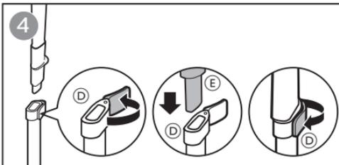
EN Hang & Lock feature and water tank must be on the same side.
