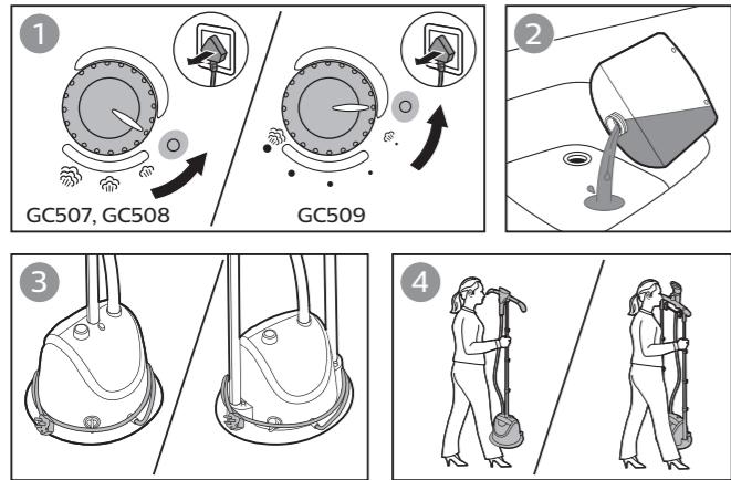
**EN** Always empty the water tank after usage, to prevent calc build-up and maintain good steam performance.
