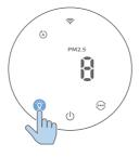
With the light sensor, the control panel can automatically turn on, turn off or dim according to the ambient light. The control panel will be off or dim when the ambient light is dark. You can touch any button to wake up all lights. Then, if no
