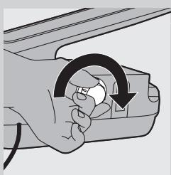
**9** Screw the Calc-Clean rinsing cap tightly back onto the steam generator.
