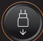
i6  | Unplug for use.                 | Unplug the appliance for use. Otherwise, it will not switch on. Only during AUTOCLEAN is it possible to have the appliance plugged in.                   |
