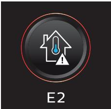
E2   | The temperature is too low.   | Make sure the temperature in the room where the appliance is used, stored, or charged is above 5 °C.
