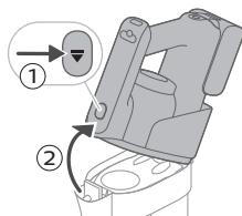
**1** Press the release button (1) to release the 3-in-1 handheld of the dust bucket and then lift the 3-in-1 handheld off the appliance (2).
