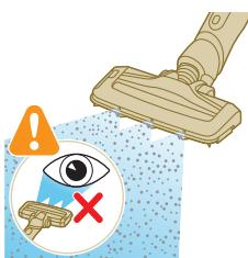
**Caution: Do not look directly into the LEDs of the LED nozzle or point the LEDs at someone's eyes. The LED light is very bright.**
