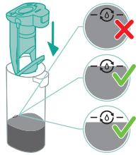
**i** Note: If the dirty water level is below the AUTOCLAN level, it is not necessary to empty the tank before starting the AUTOCLAN program. You can skip the following steps and move forward to step 6.
