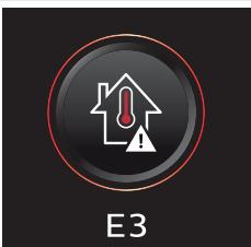
E3  | The temperature is too high.  | Make sure the temperature in the room where the appliance is used, stored, or charged is below 35 °C. Do not expose the device to direct sunlight or high temperatures (near hot stoves, in microwave ovens, or on induction cookers). Batteries may explode if overheated.
