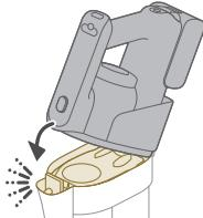
**⚠ Caution: Do not reconnect the 3-in-1 handheld to the dust bucket without the filter case being inserted in the dust bucket.**
