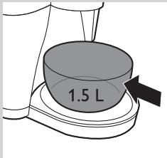
**7** Place a bowl with a capacity of 1.5 litres on the drip tray cover.
