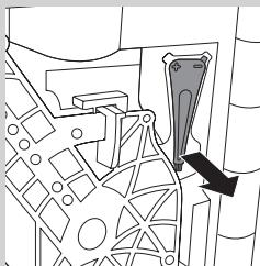
Over time the grinder may change to a coarser setting. It is recommended to adjust the grinding degree when you notice this. These adjustments are not required regularly.
