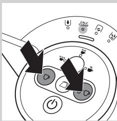
**8** Press the 1-cup button and the 2-cup button simultaneously for 1 second to start the descaling procedure.
