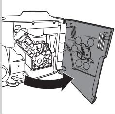
**4** Press the PUSH button (1) and pull at the grip of the brewing unit (2) to remove it from the coffeeemaker.
