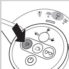
**4** Press the 1-cup button to start the rinsing cycle.
