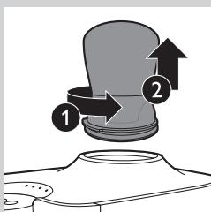
**2** Turn the bean-funnel anticlockwise to remove it.
