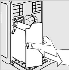
**6** Remove the water tank by pulling the handgrip.
