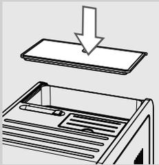
**3** After removal put the protection cover on the machine to prevent dust.
