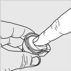
**23** Reassemble the lid. Make sure that you press it in the middle to have it correctly inserted.
