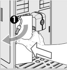
**5** Push gently on the edge of the water tank door to release the handgrip.
