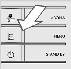
**3** Press the "☰" **MENU** button to scroll the functions until displaying the coffee temperature management function.
