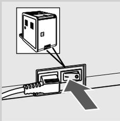
**13** Switch the power button to "I" to turn on the machine. The red led next to the "I" button blinks.
