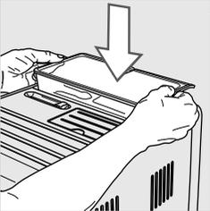
**4** Insert the coffee bean hopper into the compartment as shown on the image.
