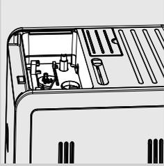
To remove the tray push the hooks on the bottom of the coffee bean hopper. This is shown in the picture on the left.
