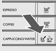
**2** Press the “☞☕” button. The machine shows this display.
