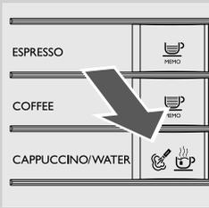
**7** Press the “☕” button. The machine shows this display.
