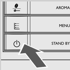
**14** To turn on the machine, simply press the "I" button. The control panel indicates that the circuit must be primed.
