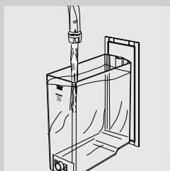
**11** At the end, fill the water tank again up to the MAX level. Now the machine is ready for coffee brewing. You will see the display as shown at the left.
