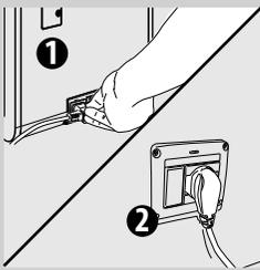
**11** Insert the plug into the socket located on the back of the machine.
