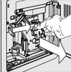
**4** To remove the brew group, press the «PUSH» button and pull it by the handle.
