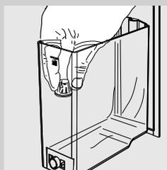
**1** Remove the small white filter from the water tank and store it in a dry place.
