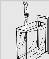
**18** When the water tank is empty, remove the water tank, rinse it and fill it up to the MAX level with fresh water. Place it back into the machine.
