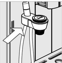
**10** For storage you can put the suction tube as shown in the picture.
