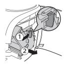
**4** Press the PUSH button and pull at the grip of the brew group to remove it from the machine.
