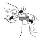
To detach the automatic milk frother, press the sides (1) and remove it by pulling it out while making slight lateral movements (2).
