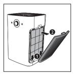
7 Repeat the above steps and assemble the air purification filter for the other side of the appliance.
