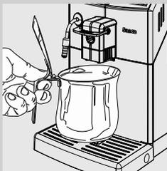
**1** Place a container under the dispensing spout to catch the small amount of water which will be dispensed.
