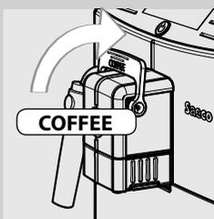
**1** Push the lever upwards to select the “COFFEE” function.
