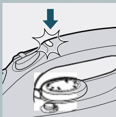
If the Auto-shut-off is activated (red pilot light blinks), move the iron slightly to deactivate it (blinking stops).
