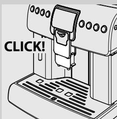
*Note: Before any brewing procedure and/or when bringing the dispensing spout back to its normal brewing position, make sure that it is correctly positioned. This can be noted through the CLICK indicating the correct position. If this is not done, some product might leak out of the dispensing spout.*
