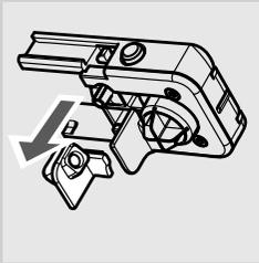
**13** Remove the suction tube joint from the Cappuccinatore.
