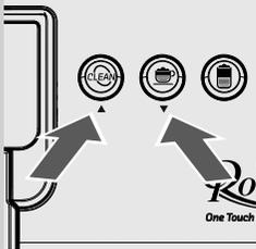
At first start-up, the machine requires you to select and store the desired language for the displayed messages. This allows you to adjust the parameters of the beverages to the typical parameters of the country where the machine is used. This is why some languages are differentiated also by country.
