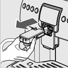
**7** Only once the cycle is complete press the side buttons and remove the Cappuccinatore.
