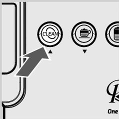
**8** With the machine on, press the "CLEAN" button.
