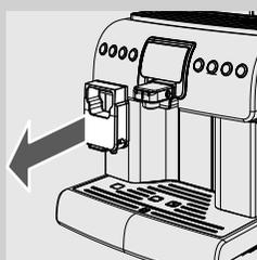
*Note: Keep the suction tube removed from the Cappuccinatore while the descaling cycle is performed.*
