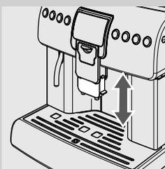
Most cups on the market can be used with this coffee machine. The height of the dispensing spout may be adjusted to better fit the dimensions of the cups that you wish to use.
