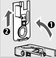
**11** Rotate and lift the Cappuccinatore cover and remove it from the Cappuccinatore body.
