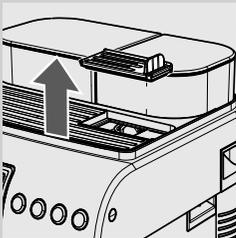
Pre-ground coffee must be poured into the relevant compartment positioned next to the coffee bean hopper. Only use ground coffee for espresso machines and never coffee beans or instant coffee.
