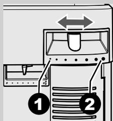
To make any adjustment, use the lever located on the side of the machine. Turn the lever one notch at a time and brew 2-3 cups of coffee; this is the only way to notice differences in grind.
