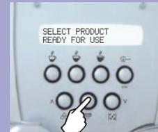
Press the "OK" button to restore the machine to normal operation.
