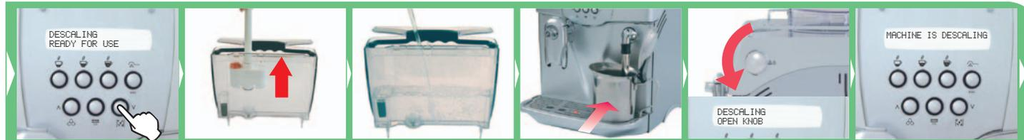
When the machine gives the signal, press the button x 5 seconds.
