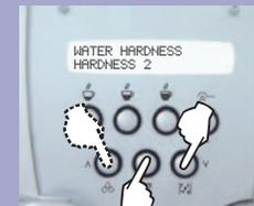
Select the corresponding hardness (e.g. 2 squares = Hardness 2) and memorize the value by pressing the "OK" button.
