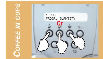
Place a cup beneath the brew unit, press the button corresponding to the type of coffee desired and **keep it pressed while coffee is being dispensed.**
