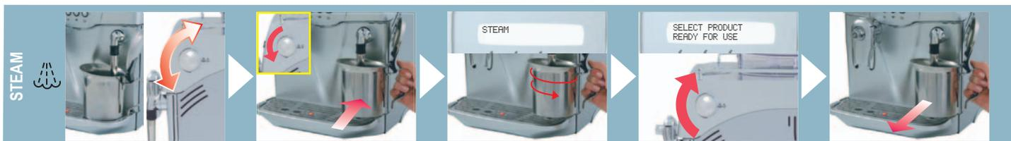
Open the knob to discharge any residual water. Close the knob.
