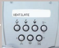
A message is displayed indicating that the machine circuit needs loading.
