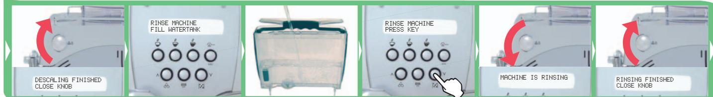
When the descaling cycle is completed, close the knob.
