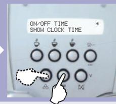
Menu for programming machine ON/OFF times.
